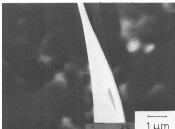
FIGURE 3 SEM picture of whisker-800 synthesized in Ar/H 2 atmosphere.
